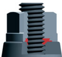
Nut in braced condition. Metal head support for high preload-force. Tight in both the thread and nut bearing face.
