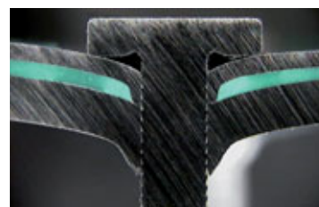
Steel sheet/ Steel profile with adhesive
