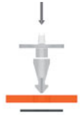
3. Feed the fastener pin through the hole, optionally secured against loss by a retaining washer.
