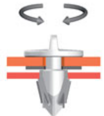
5. To open the fastener, a quarter-turn to the left or right will stretch the elastic part of the cage and release the fastener pin.
