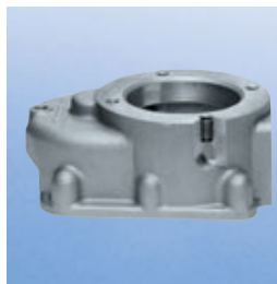
Cast aluminium gear box housing. Tang removal challenging due to heavy workpiece.
