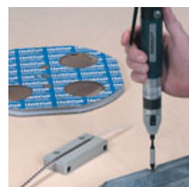
Installation of HELICOIL® plus
