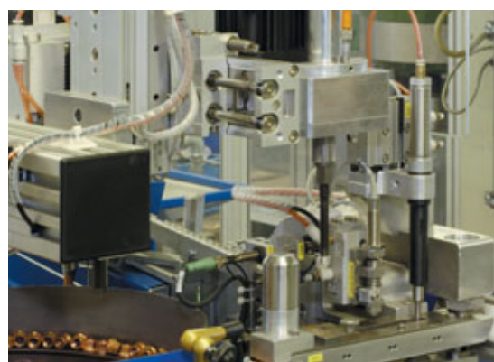
Automatic installation of HELICOIL® plus screwlock, separation by vibration.
